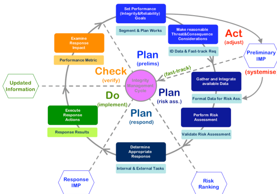
Figure 1. Pipeline Integrity Management Cycle
